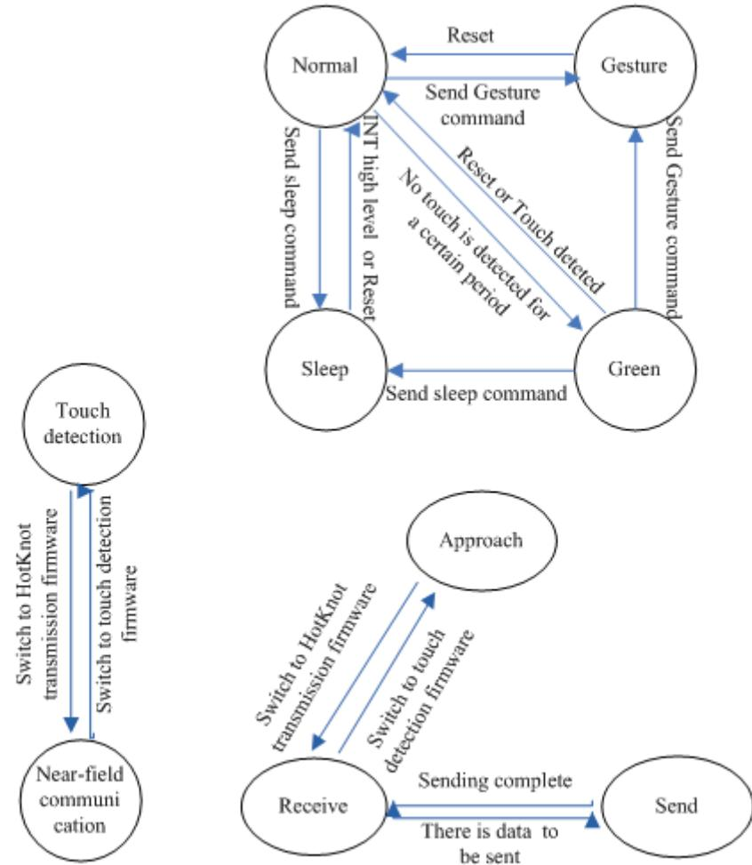
GT911 can switch between Normal mode and Low Power mode automatically by default. When touch is pressing down or after touch is released for a certain period (0s ~ 15s, configurable), GT911 operates in Normal mode. If no touch is detected within that period, GT911 enters Low Power mode (low-speed scan).
