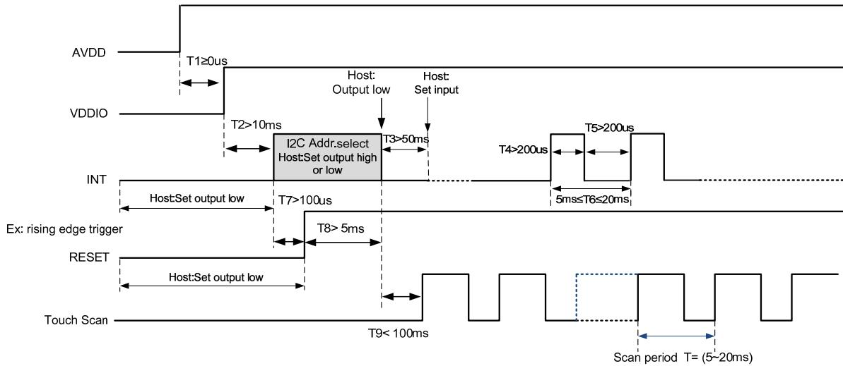
Whether host outputs high or low after INT T2 depends on which I<sup>2</sup>C slave device address the host employs to communicate with GT911. If the address is 0x28/0x29, host outputs high; if the address is 0xBA/0xBB, host outputs low.
