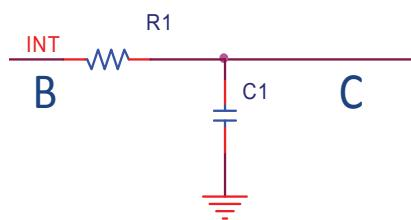
Connect B to GT911 INT and C to host INT; pull-up resistor connected to host INT is not required.
