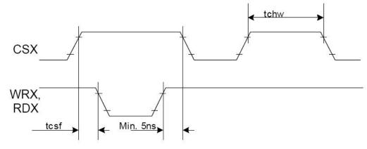
Note: Logic high and low levels are specified as 30% and 70% of IOVCC for Input signals.
